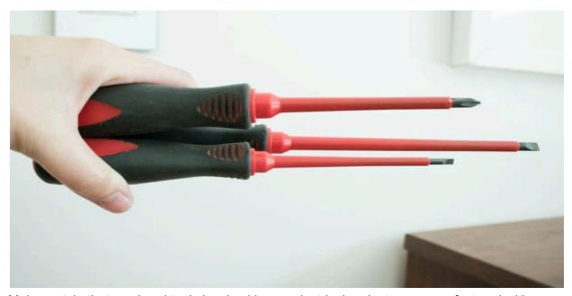
Make certain that any hand tools involved in any electrical projects are manufactured with insulated handles. These products are highly regulated for safety, as the cushioned handle will help protect you against shock. Brands are required to include an official 1,000-volt rating symbol on products that pass the test, so keep and eye out for it and choose a qualified tool for your job.
